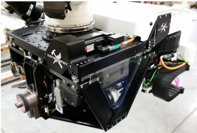
Figure 2. Electroimpact multi-function end effector
