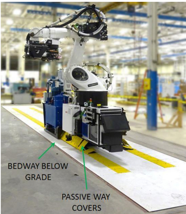
Figure 11. Electroimpact flush floor bedway system with passive way covers
