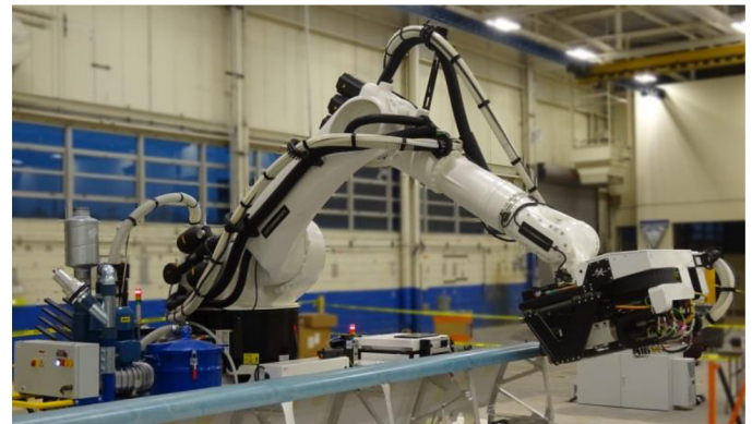
Figure 3. Automation "clamped" against [test] work piece
