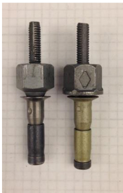
Figure 8. BACB30VK twist-type blind bolts
